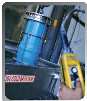
Hydrostatic Pressure Test
