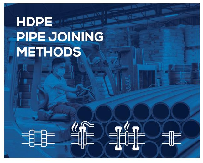
PE pipe or fittings are joined to each other by heat fusion or with mechanical fittings. PE pipe may be joined to other pipe materials by means of compression fittings, flanges, or other qualified types of manufactured transition fittings. There are many types and styles of fittings available from which the user may choose. Each offers its particular advantages and limitations for each joining situation the user may encounter.
